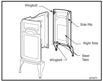
Fig. 4 Attach right side to rear skirt.
